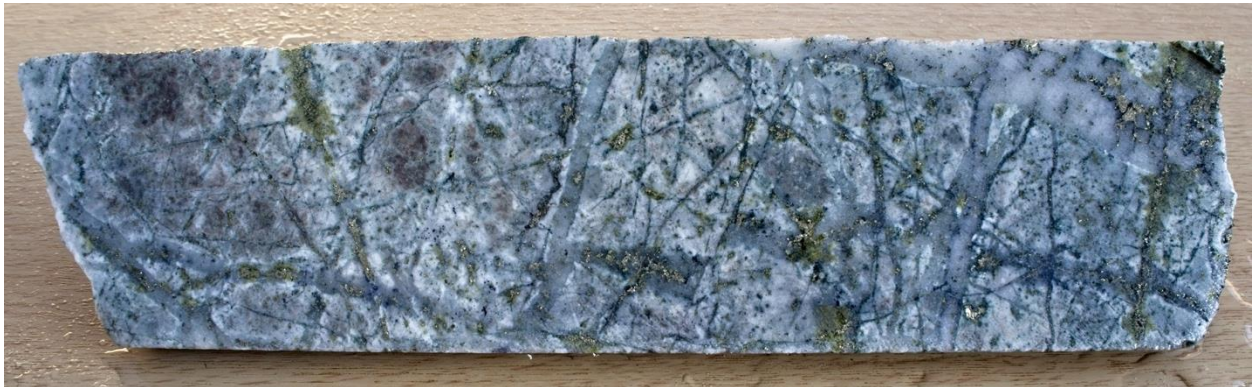
Figure 18. ELID019, 241.15m from a sample interval reporting 0.62% Cu, 0.032% Mo, 4.4 g/t Ag. Intense, multiple generations of A-type veins in feldspathic arenite host rock. The A-type veins contain an assemblage of pyrite-chalcopyrite-molybdenite with minor magnetite. Chalcopyrite is also introduced by green mica veinlets containing chlorite, epidote with chalcopyrite and pyrite. Core is HQ diameter (63.5 mm).
