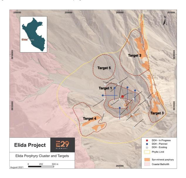
**Figure 2**. Target 1 showing existing and planned drill holes. The horizontal projection of mineralized intervals is shown as grey bands on the existing drill holes.
