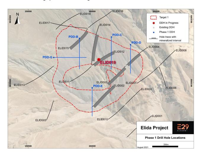
**Figure 3**. An oblique view of Target 1 with red shading showing the interpreted position of coppermolybdenum mineralization projected to surface in relation to drill hole ELIDO19, which is currently in progress. The centre of the ring of mineralization is occupied by an early-stage mineral porphyry intrusion. The interpretation is based on alteration and mineralization exposed by drainage incisions and drill holes.
