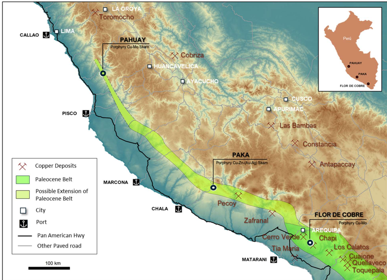
Figure 13: Location map for the Flor de Cobre, Paka and Pahuay Projects. The light green tone is the approximate position of the Paleocene Magmatic Arc and the Southern Peru Copper Belt, which hosts major porphyry copper deposits in the region.
